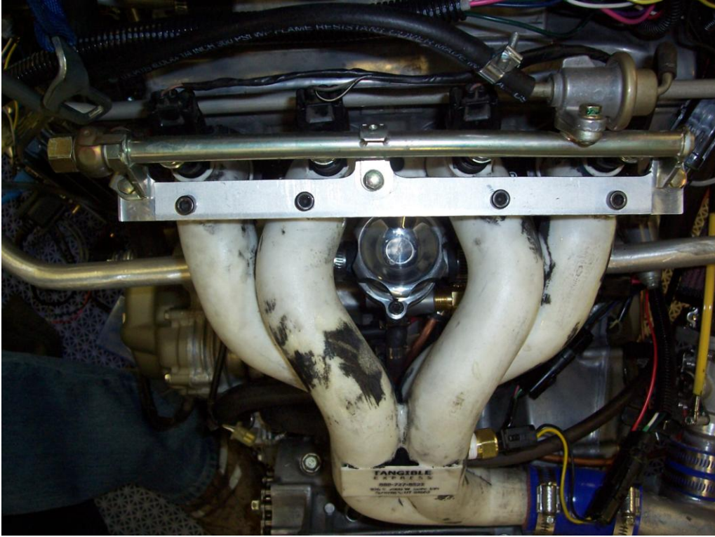
Figure 8 – A top view showing better the access allowed for refilling the coolant system. Notice the injectors are placed on the top of each port directly inline with the port in the head.
