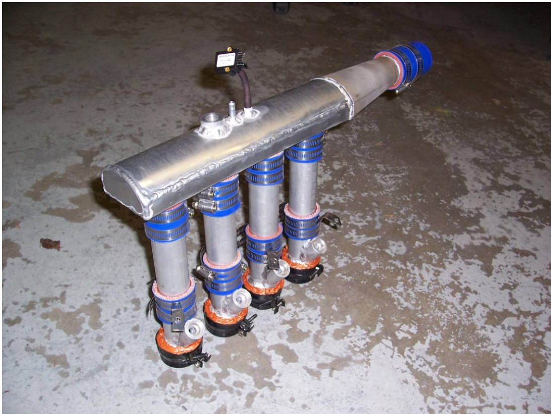
Figure 3 – The aluminum log plenum intake. Notice the angle of the injectors mounted just above the rubber boots.
